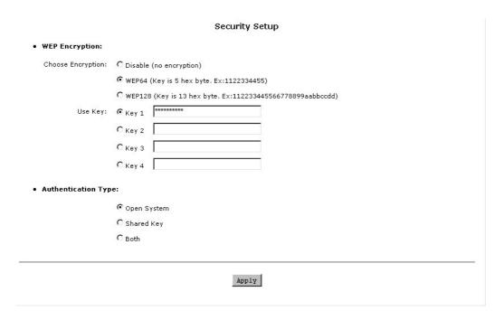
The IIMbps Wireless Access Point allows you to create 4 data encryption keys to secure your data from being eavesdropped by unauthorized wireless user. To activate and set the WEP keys, please do the following:
